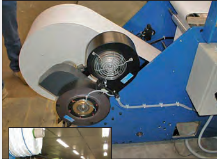
Zugregelung an einer Flexo-Druckmaschine Tension control on a flexographic printing machine
