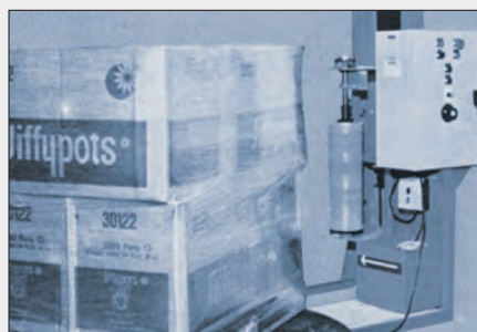
Zugregelung an Palettenverpackmaschine Tension control at pallet packing
